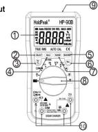
①LCD Display: 6000 digits, full function symbol display ②SELECT key:This key work on the "CAP➡ ③Ω" range , Push the key to choose resistance, diode ,continuity test, on the voltag or current range, change to DC/AC, and  $^{\circ}\mathbb{C}/^{^{\circ}}F$  range , change to  $^{\circ}\mathbb{C}/^{^{\circ}}F$
